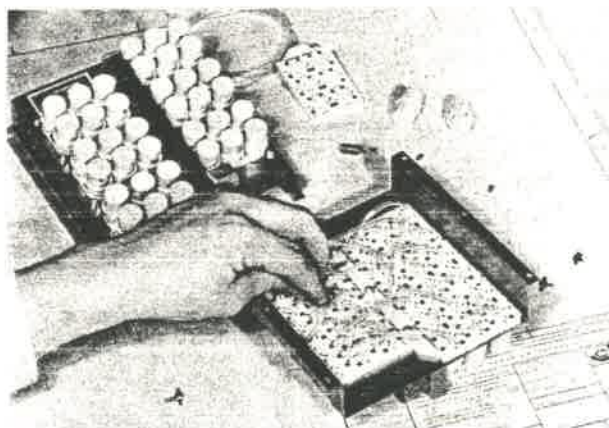
Typical Fluidic Circuit Construction Using F-3702-251 NOR Logic Element and other Air-Logic Standard Fluidic Components
